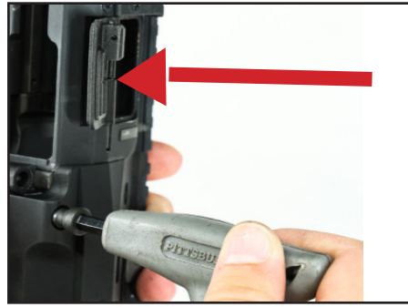
Figure 16: Remove the handguard retainer screw
