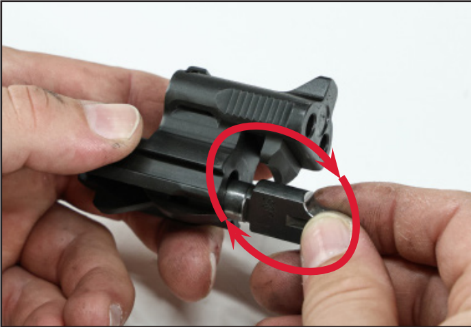
Figure 31: Inserting the locking piece
