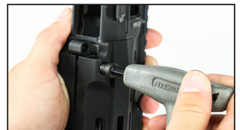
Figure 35: Put the handguard retainer screw
