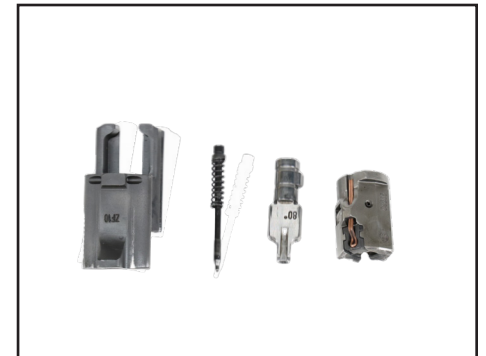
Figure 21: Disassembled bolt group
