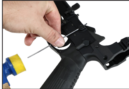
Figure 23 Step 3: Removing the ejector axle retainer
