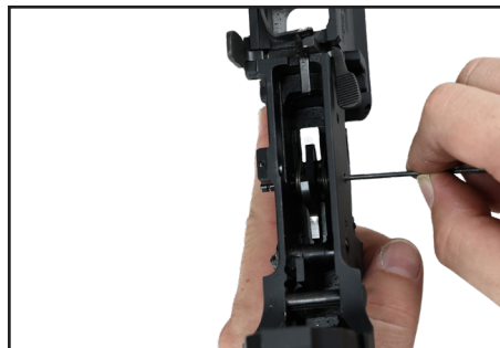
Figure 29 Step 8: Drift the trigger pin
