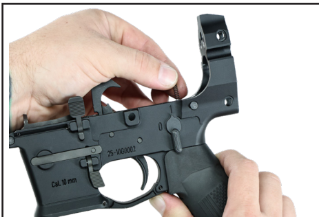
Figure 25 Step 6: Removing the ejector spring
