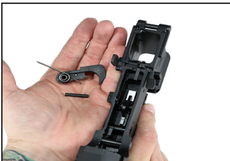
Figure 28 Step 7: Removed the hammer and ham- mer spring
