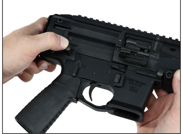
Figure 37: Pushing the takedown pin
