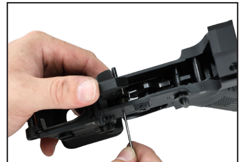
Figure 27 Step 7: Drifting the hammer pin
