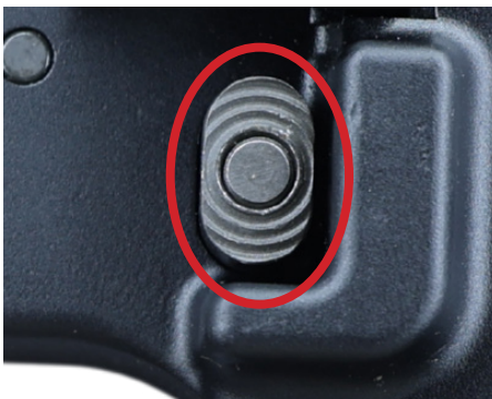
Figure 3: Magazine release button
