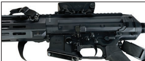
Figure 7: Mounting the carrying sling to the ZF-56
