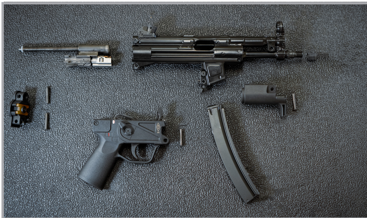
Figure 23: ZF-5P/ZF-5T/ZF-5K assembly groups
