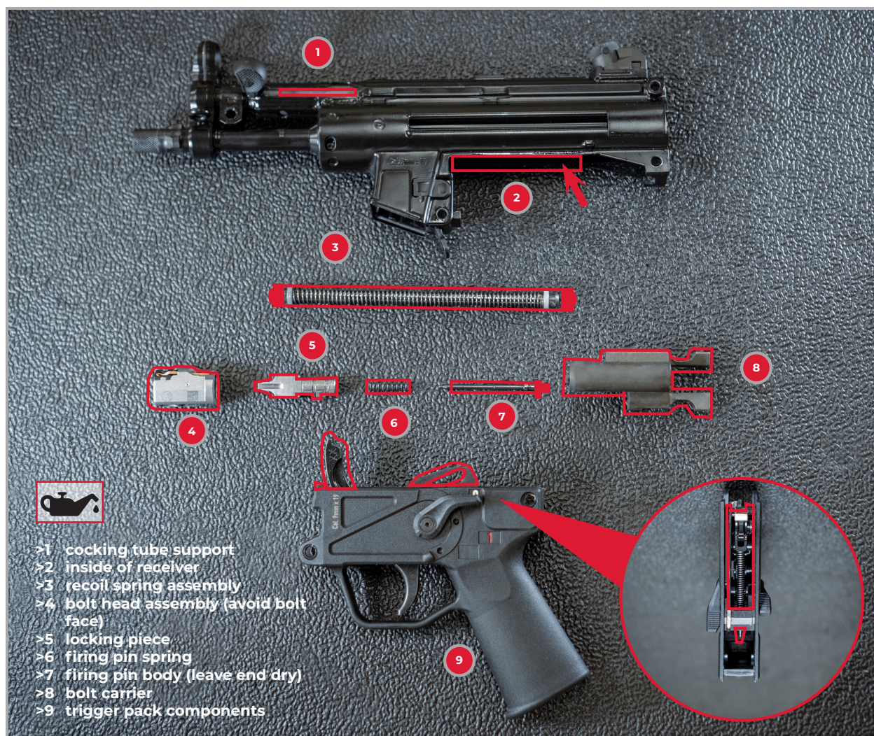
Figure 37: ZF-5P/ZF-5T/ZF-5K lubrication points
