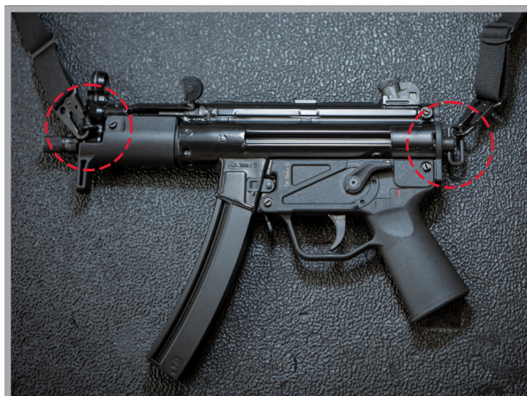
Figure 7: Mounting the carrying sling to the ZF-5P/ZF-5T/ZF-5K (2 point configuration)
