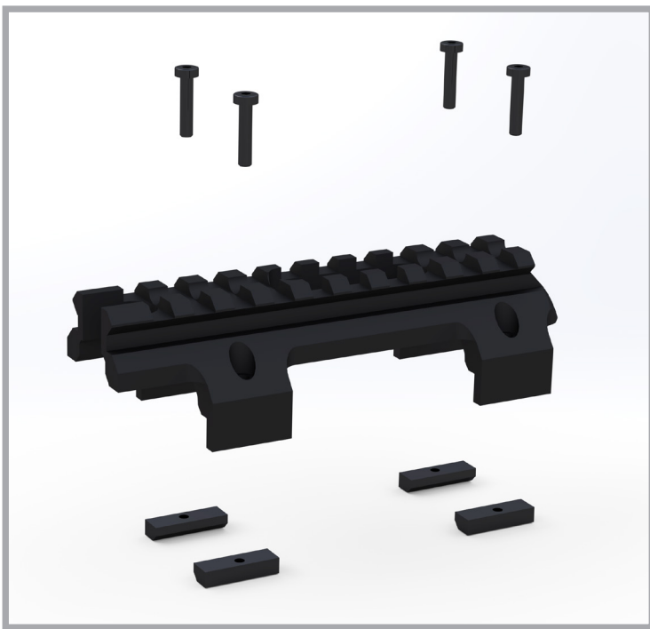
Figure 9: Mounting the Picatinny optic rail
