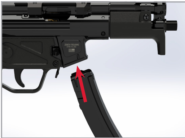
Figure 17: Inserting the magazine
