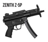
CALIBER 9 x 19 mm Parabellum OA LENGTH 13.7 inches BARREL LENGTH 5.8 inches BARREL cold hammer forged 32 chrome molybdenum vanadium WEIGHT EMPTY 4.6 pounds OPERATION semi-automatic, roller-delayed blowback
