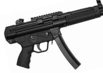
CALIBER 9 x 19 mm Parabellum OA LENGTH 17.9 inches BARREL LENGTH 8.9 inches BARREL cold hammer forged 32 chrome molybdenum vanadium WEIGHT EMPTY 5.5 pounds OPERATION semi-automatic, roller-delayed blowback TWIST RATE 1:9.8 SIGHTS rear drum for elevation and windage, front protected post <u>CAPACITY</u> 30 COLORS black ADDITIONAL barrel has 3-lug quick attachment and 1/2 x 28 threaded end
