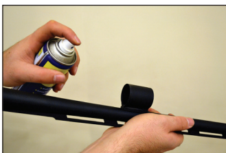
STEP 9: Clean the gas ports on the inside of the barrel lug. Clean inside of the barrel lug.
