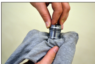
STEP 8: Clean the inside and the outside of the piston using the same method.
