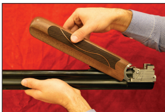
STEP 2: Detach the forearm from the barrel by lifting off.
