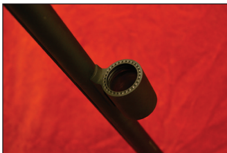
STEP 5: O-ring is located inside the barrel ring so it's not visible on the magazine tube.
