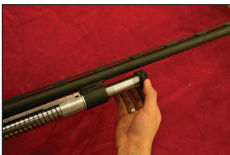
STEP 3: (G125 model only) Unscrew the supporter nut off the front of the magazine tube.
