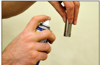
STEP 2: Clean and lightly oil choke tubes.
