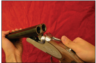
STEP 4: While keeping the top lever pushed to the right, install the barrel to the receiver at an approx 40° angle. Be sure the barrel is completely installed to the receiver otherwise the shotgun will not close.
