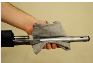
STEP 7: Push the latch under the trigger group (loading figure 2/ cartridge drop lever). Pull back the bolt handle. Clean the outer surface of the magazine tube with a soft cloth.
