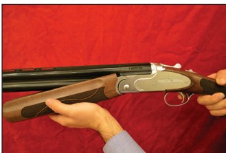
STEP 7: Mount the forearm to the barrel. Be sure the opening latch of the forearm is completely closed.
