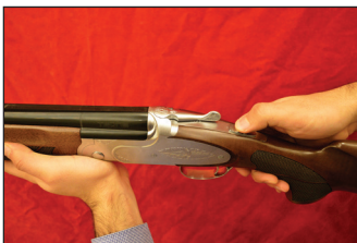
STEP 8: Put the safety on by moving the safety switch to the rear position.
