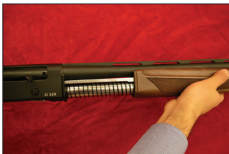
STEP 2: Remove the forearm by pushing it forward.
