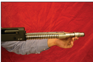
STEP 6: Slide the gas piston off the front the magazine tube.
