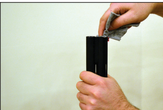
STEP 3: Carefully begin threading choke into shotgun and tighten until snug. Check choke occasionally to ensure it has remained tight after shooting.
