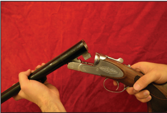
STEP 3: Push the top lever fully to the right.
