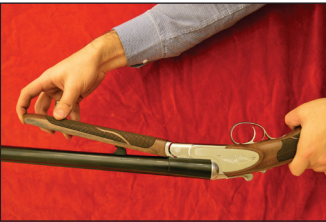
STEP 5: Mount the forearm to the barrel. Make sure that the opening latch is completely closed.
