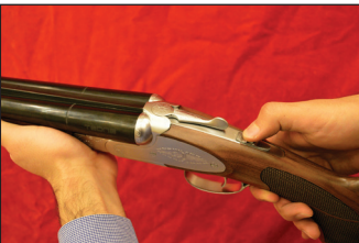
STEP 5: Mount the forearm to the barrel. Make sure that the opening latch is completely closed.
