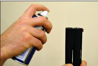
STEP 1: Clean and lightly oil the choke threads in barrel.
