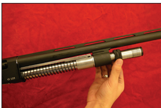
STEP 3: (G125 model only) Unscrew the supporter nut off the front of the magazine tube.
