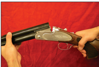
STEP 6: Lift the barrel upwards to close the shotgun, be sure the barrel and receiver are properly aligned and the top lever returns slightly to the right of center. It is normal that the top lever does not return exactly to the center, this allows for wear.
